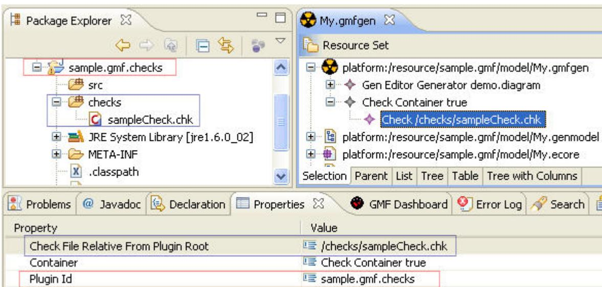
**Figure 10.5. Adding a new check file**
